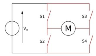
This is equivalent to the circuit above, but it has switches instead of transistors. What would happen if we closed switch 1 and 3? 2 and 4? 1 and 4? 3 and 2? lets make a table:
