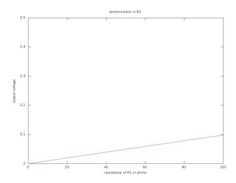
As you can see here, the difference in voltage is .1 v, but it is very linear. This is the case where R2=5000 ohms. You can imagine this can be frustrating, because on one hand you want a linear system, but on the other, you want a wide delta V.
