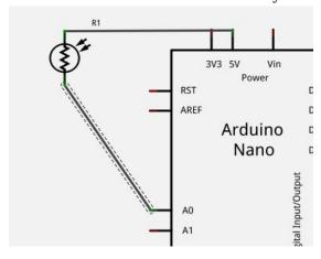
We see here that some fool has hooked the photoresistor up to 5V and an input pin. We know that:
