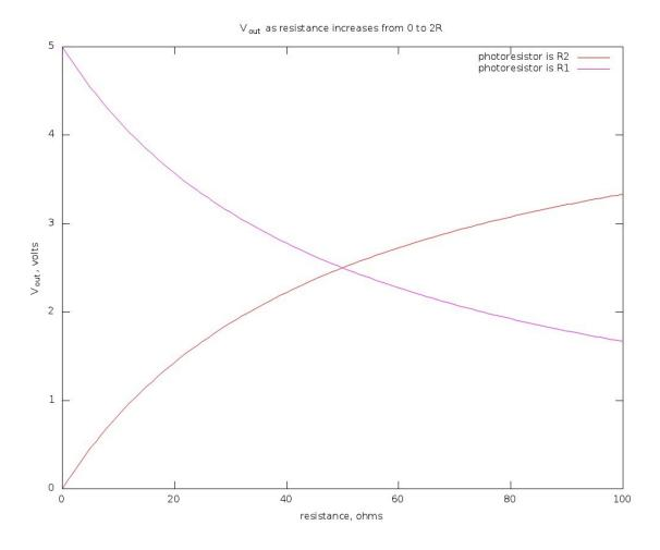
However, if we do something like make the other resistor much larger (1-2 orders of magnitude) we can make it much more linear. This is because as the other resistor gets bigger, the change that the photoresistor creates is much smaller. Of course, this means that the range that you can read in is smaller:
